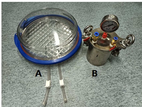
A: MIC Cultivation System; B: 304 Stainless Steel Tank Cultivation System
